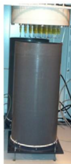
Fig. 1. Column of soil under rain simulator
