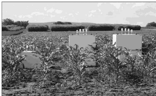
Figure 1: Manual chamber measurement system to determine N 2 O fluxes.
